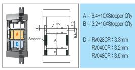
Stoppers control divider position and lock the dividers into place during operation.
