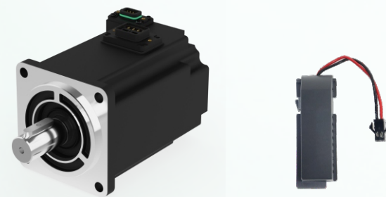
Multi-turn absolute encoder with external battery power supply can still remember the position when the drive is powered off
